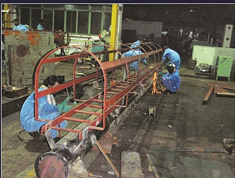
Fabrication of Fore Mast at Shore-Workshop
