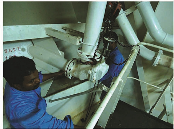
Dismantling of storm valve at anchorage
